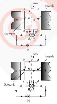
Principle: When a coil carrying current is placed in a magnetic field, it experiences a torque. As a result of this torque, the coil begins to rotate.
