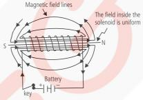
**2. (d)**: The magnetic field inside a current-carrying solenoid is constant in magnitude and direction, and acts along the axis of the solenoid.
