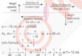
Spherical lens is convex lens or converging lens of focal length 12 cm.
