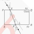
As can be seen that at point X and X', the incident ray, the refracted ray and the normal all lie in the same plane.
